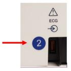
A number 2 circular label on the back housing of the ELI electrocardiograph located next to the ECG input connector indicates the electrocardiograph internally contains a version 2 UTK.
