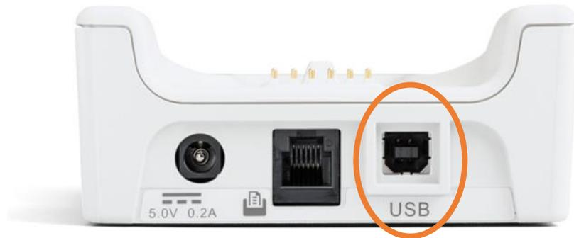
The MicroTymper 4 unit must be placed in the cradle for data to be transferred. The cradle must be plugged into power and the device should be turned on. The transfer of data is initiated from the TympView program running on the PC.
