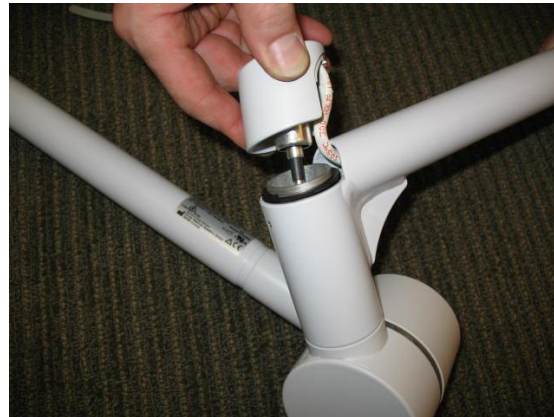
Replace plastic cap/electrical connector and secure with screw
