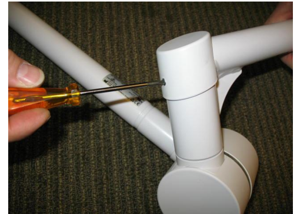
Replace plastic cap/electrical connector and secure with screw
