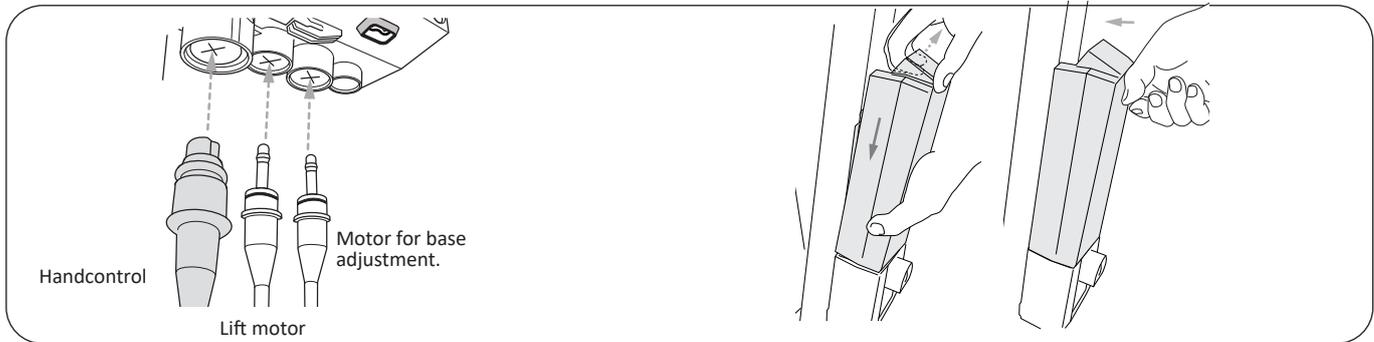
4. Connect cables to the control box, see illustration. Make sure plugs are fully seated.
